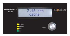
The model UV-100 ozone analyzer is for general purpose measurement of ozone in air. Its range is .002-100 ppm (v) with 2% accuracy, and it includes a built-in data logger. The UV-100 weighs only 2.1 kg (4.7 lb), it is powered by an AC adapter or 12 V external battery, and is equally versatile for the laboratory
